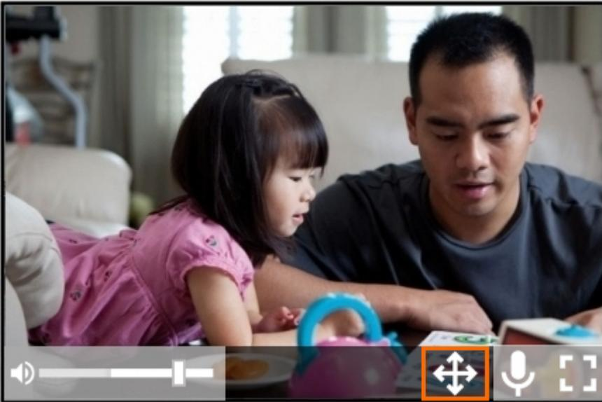
4. PTZ control appears in the middle of the image and your mouse pointer becomes a small point. Click the camera image and keep your left mouse button pressed to control the camera. The camera image moves in the direction of the point. The further away from the PTZ control you click, the faster the camera moves.
