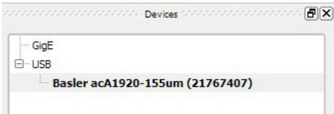
4. Under **Features**, open the item **Basler acA1920-155um** and choose the settings you would like to change. For details, see the corresponding settings in [Configure the cameras](#) in [Set up GigE cameras](#).
